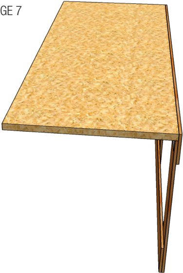
Above image shows 1/2" plywood sitting flush on frame.
