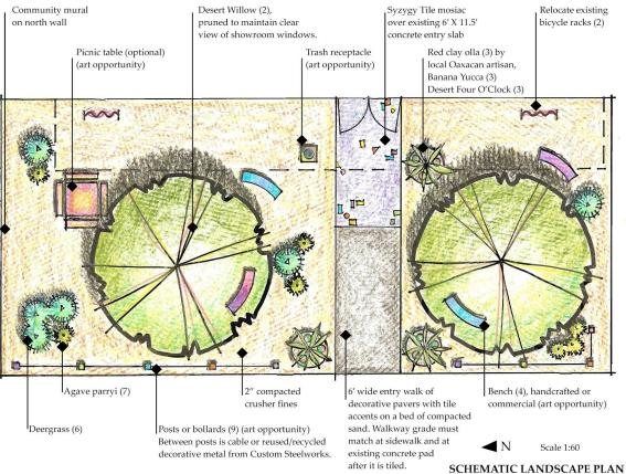
**NOTE:** Remove wheelstops and all existing paving except 6' wide concrete entry pad. Grade to detain rainwater runoff in treewells, then to overflow to street. Finish grade after compacting crusher fines to 2" layer should match sidewalk and entry walk grades where they meet.
