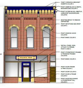
01 PROPOSED FACADE - NORTHEAST ELEVATION
